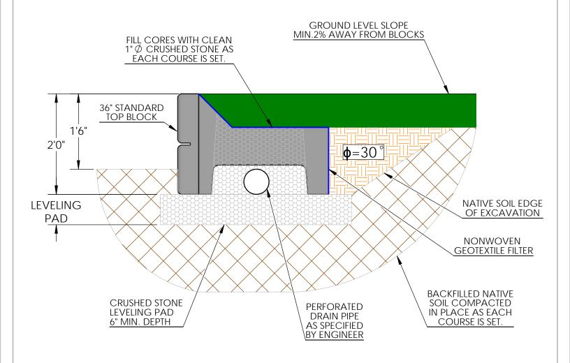
Note: This drawing was prepared by Verti-Crete, LLC for estimating and conceptual design purposes only. All information in believed to be true and accurate; however Verti-Crete, LLC assumes no responsibility for the use of this drawing for actual construction. Determination of the suitability of each drawing is the sole responsibility of the user. Final designs for construction purposes must be performed by a registered Professional Engineer, using the actual conditions of the proposed site.
