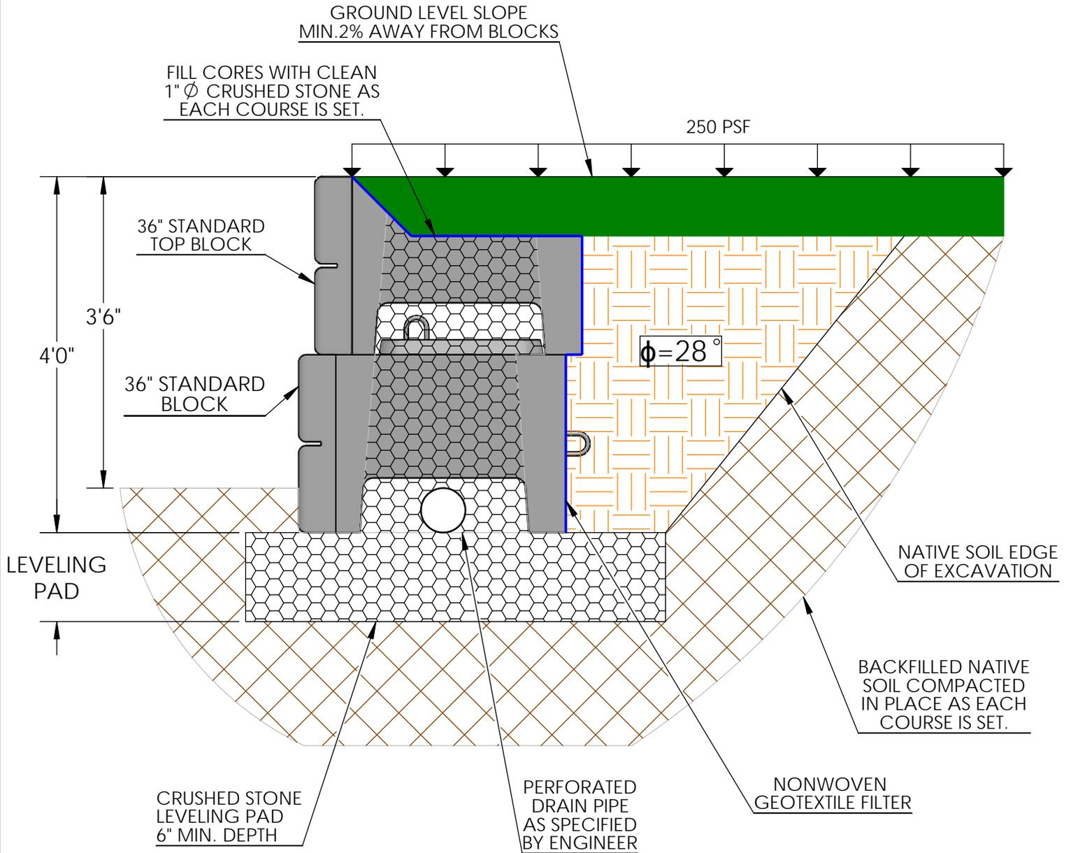
Note: This drawing was prepared by Verti-Crete, LLC for estimating and conceptual design purposes only. All information is believed to be true and accurate; however Verti-Crete, LLC assumes no responsibility for the use of this drawing for actual construction. Determination of the suitability of each drawing is the sole responsibility of the user. Final designs for construction purposes must be performed by a registered Professional Engineer, using the actual conditions of the proposed site.
