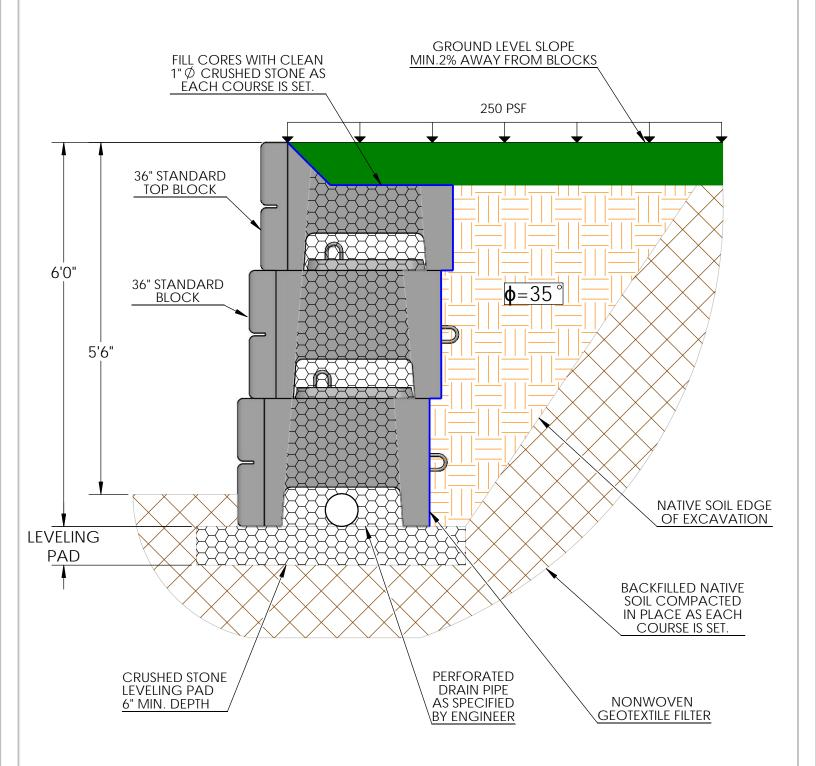
Note: This drawing was prepared by Verti-Crete, LLC for estimating and conceptual design purposes only. All information in believed to be true and accurate; however Verti-Crete, LLC assumes no responsibility for the use of this drawing for actual construction. Determination of the suitability of each drawing is the sole responsibility of the user. Final designs for construction purposes must be performed by a registered Professional Engineer, using the actual conditions of the proposed site.
