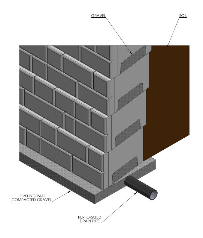
DRAIN PIPE IS PLACED INSIDE THE COMPACTED GRAVEL OF THE LEVELING PAD
