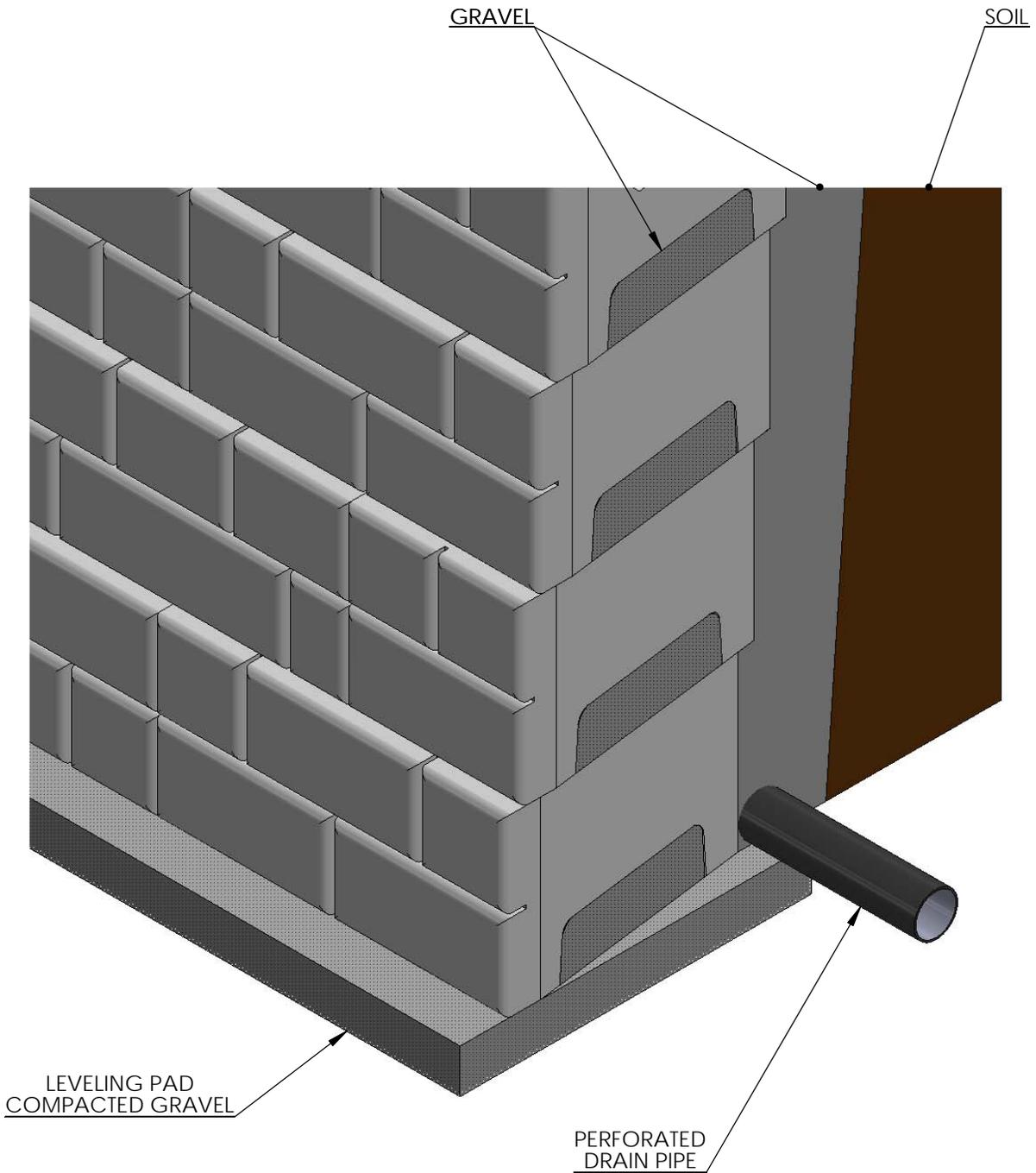
DRAIN PIPE IS PLACED BEHIND THE BLOCK AND ON TOP OF THE LEVENING PAD.
